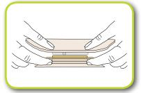
Start at bottom and apply pressure completely around the flanges until the pouch and flange are snapped completely together.
